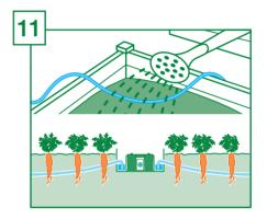
Position your capillary matting. For best results ensure that the matting slopes slightly downwards as it runs away from the AQUAbox. This eases the flow of water/nutrient solution.
