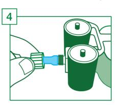
Attach the AQUAvalve to the end of the 9mm pipe that you pushed into the Body.
