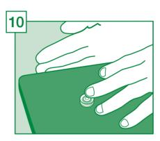
Seat AQUAbox in centre of mound created in Step 1. Push the circular spirit level into the lid of the Body.
