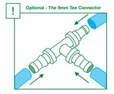
Use the 9mm tee connector to run additional AQUAboxes from the same reservoir. This is easily done during setup. If adding to an in-use system ensure your reservoir is switched off. Cut your 9mm pipe at an appropriate point and join the cut lengths to the tee. Attach your additional AQUAbox to the spare connection on the 9mm tee connector.
