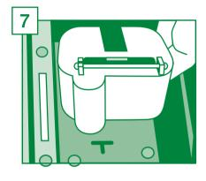
Align the 'half moon' section on the rear of the AQUAvalve with the 'T' section in the AQUAbox Straight Body.
