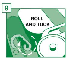
Tightly roll both inside ends of the capillary matting and tuck into the AQUAbox alongside the AQUAvalve.
