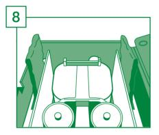
Cut your length of capillary matting into two equal pieces and thread in on both sides of the AQUAbox Straight Body
