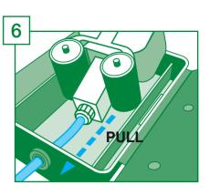
Remove any slack in the 9mm pipe by drawing excess out of the AQUAbox Straight Body.
